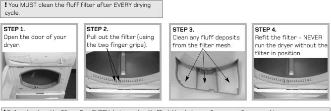
Failure to clean the filter after EVERY drying cycle will affect the drying performance of your machine.
